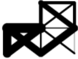
図 2: Initial configurations of 14-member trusses.
