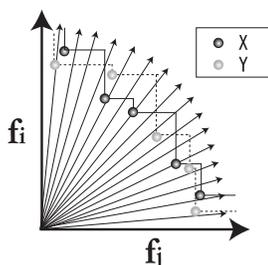
Fig. 4 Sampling the Pareto frontier using lines of intersection【LI】
