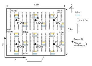
Fig. 3. Illuminance distribution measurement experiment (Plan of the room)
