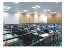
Fig. 7. Illuminance distribution measurement in Ecozzeria
