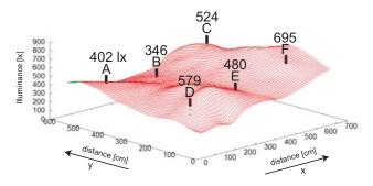
Fig. 5. Illuminance distribution (Using Intelligent Lighting System)
