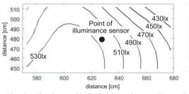
Fig. 6. Illuminance distribution in work areas (Sensor C)
