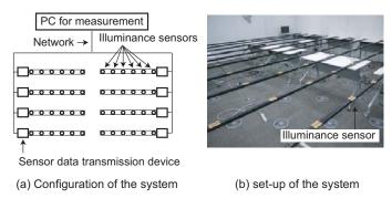
Fig. 2. Illuminance distribution measuring system
